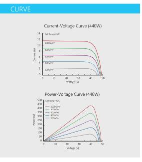
Note: the specifications are obtained under the Standard Test Conditons (STCs): 1000 W/m² solar irradiance, 1.5 Air Mass, and cell temperature of 25°C. The NOCT is obtained under the Test Conditions: 800 W/m², 20°C ambient temperature, 1m/s wind speed, AM 1.5 spectrum.
